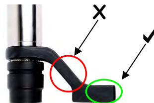
FIGURE 6 – Reaction Bar Surface
