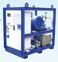
DP310E/1,000 test pump unit, pressure and speed regulated, freely programmable pressure sequence as in EN 12056-6 with data logging for test records. Interface for data transfer to external network or PC.
