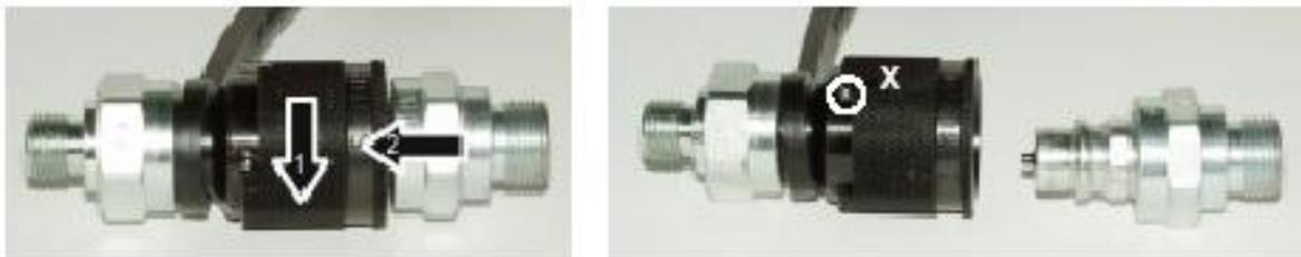
In position X, retract sleeve – plug and socket are uncoupled - the device is coupled in reverse order. The devices can only be coupled if the hose lines are **depressurized**.
