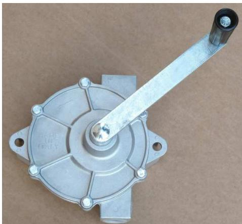
**PLINIO PUMP:** Full rotary action hand pump, self-priming, fully reversible, one revolution 360°. Cast alloy body.
