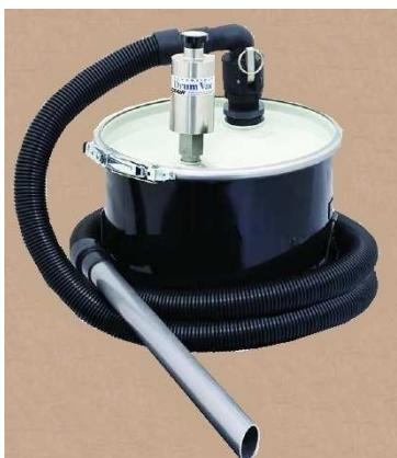
**DESMODUS:** Air operated pump, ideal for emptying the tanks of the machine tools. Single action and self priming. It works also with dirty fluid and diesel. The barrel shown is not supplied.
