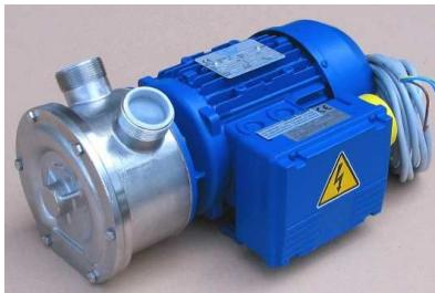
**EP NAUTIC INOX:** Liquid ring self priming stainless steel pump, two way rotation. Ideal to transfer edible liquids. Available with 230 V single phase or 400 V three phases motors.
