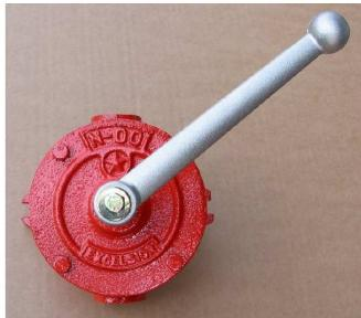
**EXCELSIOR PUMP:** Semi-rotary hand pump, self-priming, double acting and reciprocating action. Cast iron body and cover, internal parts made of bronze; according to the versions seals may be NBR (GB) or Viton (GB-be). The maximum delivery head is 25 meters. E00 version without flanges.
