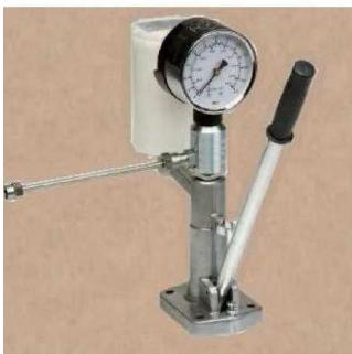
**CAR TEST PUMP:** Radiator test and fuel injector test pump, for diesel and gasoline.
