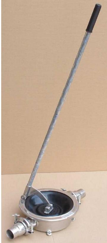
**BARADELLO JOLLY PUMP:** Hand pump with body and couplings made of stainless steel, single diaphragm, self-priming and single acting. For boats (MARINA) or liquids with suspended solids (JOLLY A / B). Available with trolley on request.
