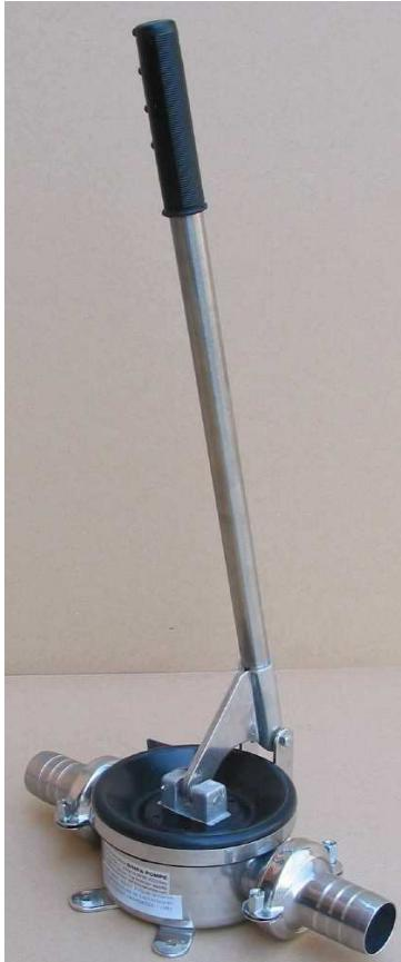
**BARADELLO JUNIOR PUMP:** Hand pump with body and couplings made of stainless steel, single diaphragm, self-priming and single acting. MARINA version is for boats. Available with platform on request.
