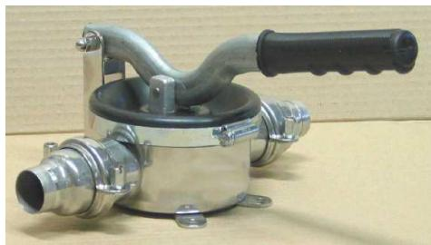
**BARADELLO MINI PUMP:** Hand pump with body and couplings made of stainless steel, single diaphragm, self-priming and single acting. MARINA version is for boats.
